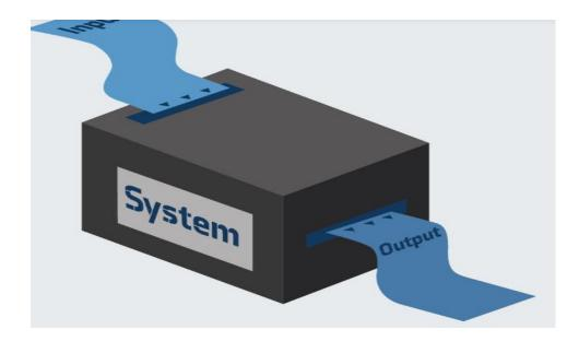
The black box in the picture represents the production system itself. On the left we have what goes into the system *(input)* and on the right is what comes out of the system *(output)*.
