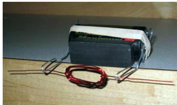
Figure 6. The complete motor setup.
