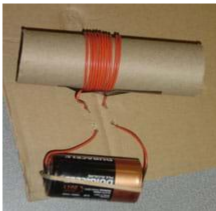
Figure 2. Setup for an Electromagnetic Field Station.
