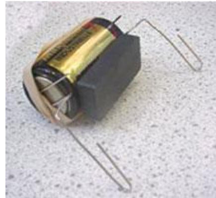
Figure 5. Battery end view, with ceramic magnet in place.
