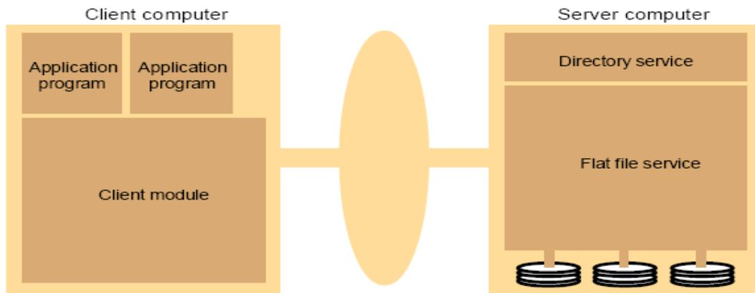
File Service Architecture : Following figure shows the architecture of file service. Client computer can communicate with server using client module to flat file service.
