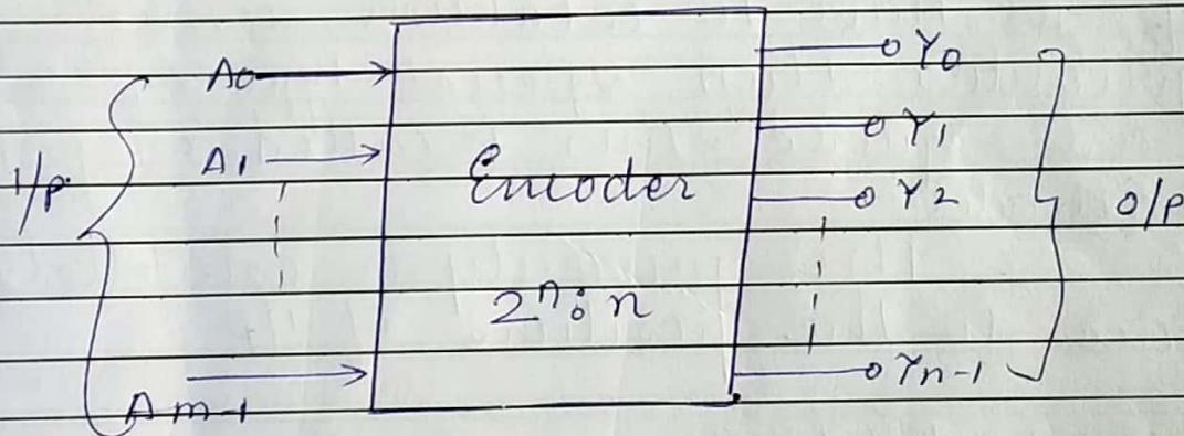
An encoder is a combinational ckt which is design to perform the inverse operation of decoder
