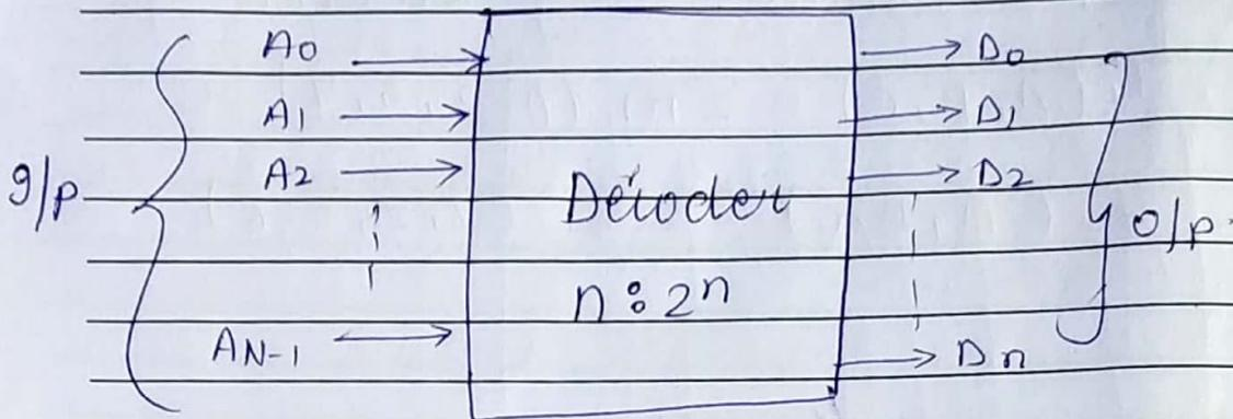
A decoder is a logic ckt that convert  $n$  bit binary i/p code into  $m$  o/p lines such that only one o/p line is activated for each one of the possible combinations of i/ps.
