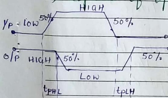
of a logic family is determined from the propagation delay. If a square wave is applied to I/P of an inverter, O/P of the inverter will be a square wave as shown in fig. It is very clear from fig that propagation delay is measured from the time difference betn 50% logic transition of I/P from its initial value & 50% logic transition of O/P. There are two types of propagation delay time  $t_{PHL}$ ,  $t_{PLH}$
