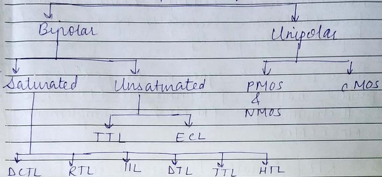
The digital logic family has broadly classified into two types namely bipolar and unipolar. The bipolar logic families are classified as saturated & non-saturated types.
