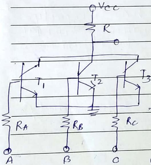
RTL ckt of three I/P NOR gate is shown in fig. In this ckt resistance is connected in series with base of each transistor to reduce hogging current effect.
