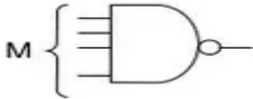
For example: A two input gate will have a fan-in equal to 2.
