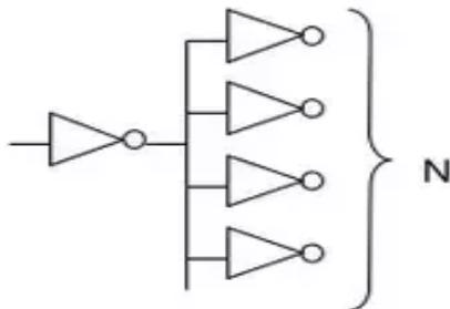
The fan-out is defined as the maximum number of inputs that can be connected to the output of a gate without degrading the normal operation.
