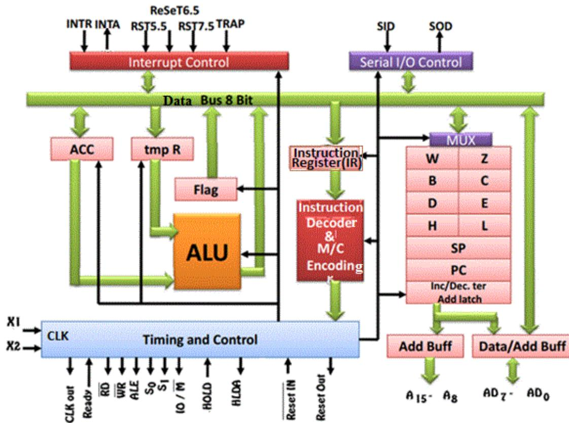
The architecture of 8085 microprocessor mainly includes the timing & control unit, Arithmetic and logic unit, decoder, instruction register, interrupt control, a register array, serial input/output control. The most important part of the microprocessor is the central processing unit.
