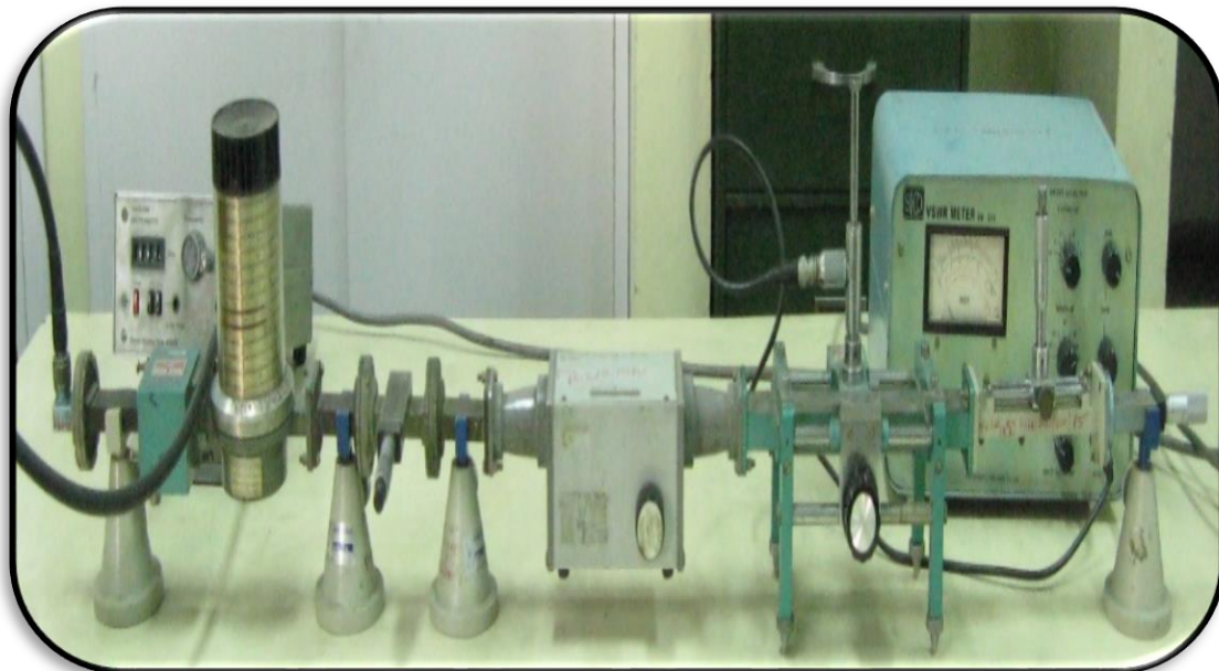
Fig.5.5.9 Measurement of VSWR on a line
