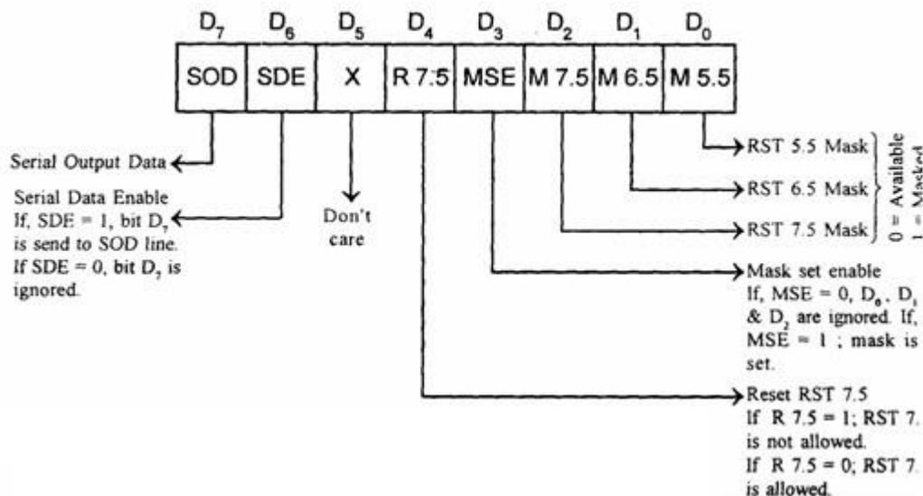
D7-D6 - The left two bits are related to the serial interface. When D6 (SDE-Serial Data Enable) is 1, then whatever is in D7 (SOD-Serial Data Output) is written to the serial data output (pin 4 of the 8085). If D6=0, nothing is written. This allows a SIM instruction to be executed altering interrupt masks without affecting serial data.
