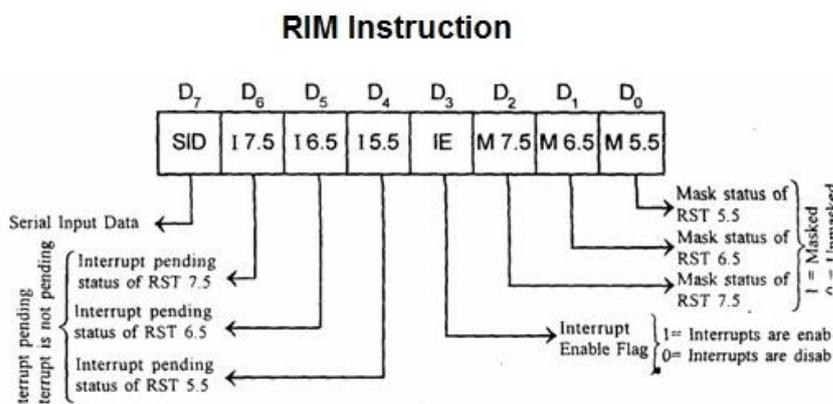
Bit D<sub>7</sub> (SID-Serial Input Data) This is the input pin of the serial data interface which is connected to pin 5 of the 8085, and indicates the high/low status of that pin.
